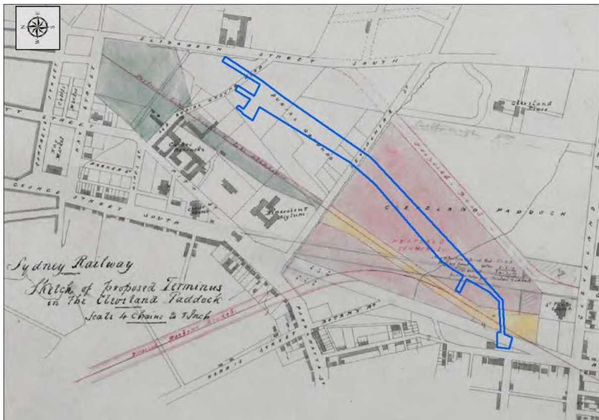
Figure 3: Plan of proposed Central railway station with Devonshire Street cemetery marked in red and the current station footprint indicated by the blue line 9
