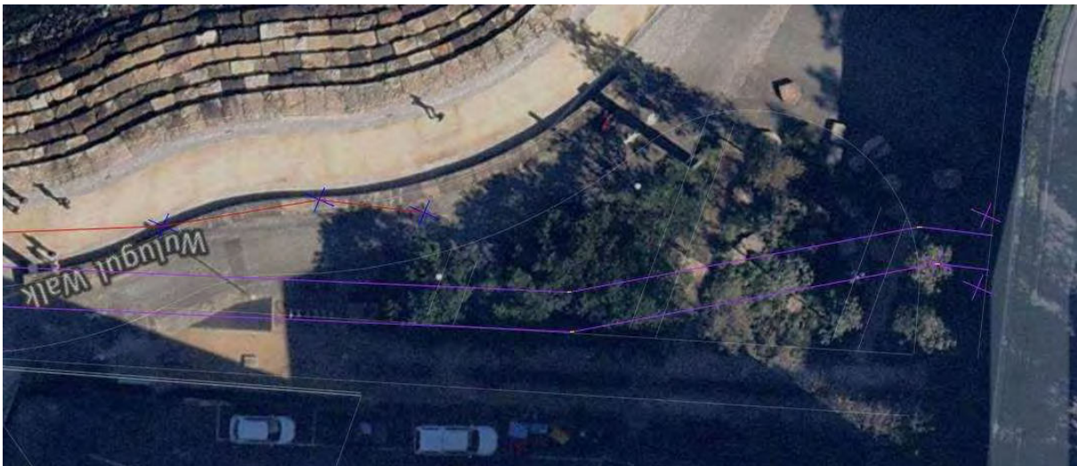
Figure 1: Snip from Nearmaps showing alignment of trench (purple)
